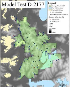
Figure 1 – Results from testing the predictive model on well and borehole data from mine permit D-2177
