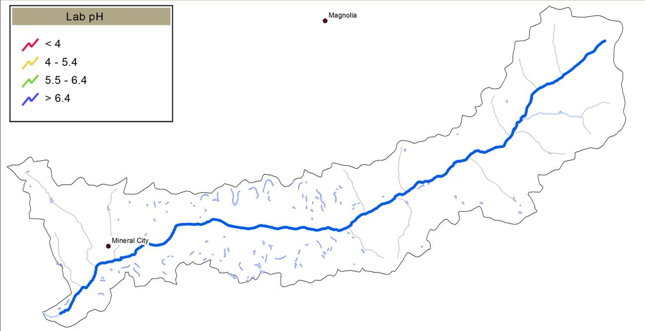
Huff Run pH values have improved from baseline conditions (1985-1998) to 2015. The entire length of Huff Run has met the pH target (6.5) for the last six years.
