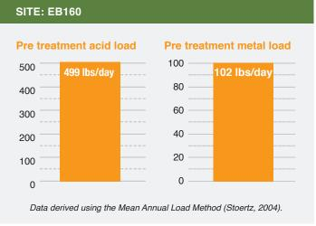
Figure 2. Estimated acid and metal loadings prior to treatment 2015
