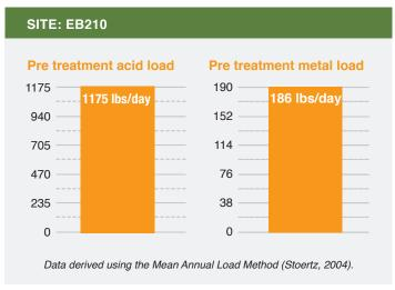
Figure 1. Estimated acid and metal loadings prior to treatment
